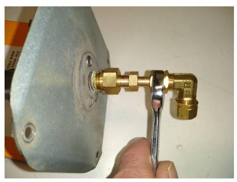
Finally tighten the large 15mm brass nut at the heater inlet.
