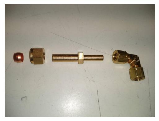
Slide the brass nut onto the larger diameter leg of the fitting. Slide the copper ferrule on after the nut.
