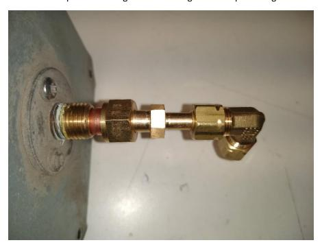
Route your  $\frac{1}{4}$ " supply tubing from your regulator and slide it into the empty socket in the  $\frac{1}{4}$ " to  $\frac{1}{4}$ " fitting. Allow the position of the fitting to self-adjust to provide the most direct routing of the supply tubing.
