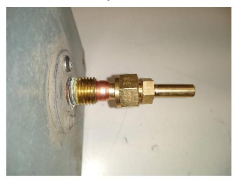
Slide the  $\frac{1}{4}$ " X  $\frac{1}{4}$ " double compression fitting onto the  $\frac{1}{4}$ " leg of the Propex fitting but do not tighten.
